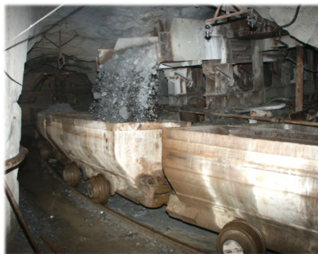
Figure 2 – Vibratory feeder of the VPR-4m type for the ore drawing and feeding from the panel to the wagons
